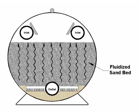
Tank Cross Section During Backwash Mode
