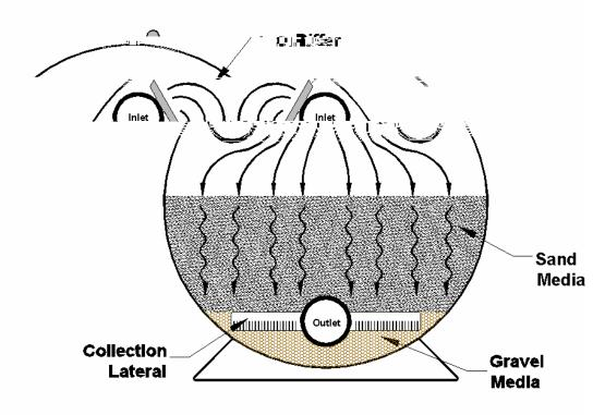
Tank Cross Section During Normal Filtration
