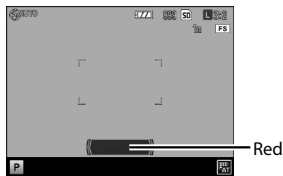
Camera is rotated too far forward or backward or unable to measure tilt.
