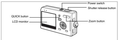
The simplest procedure for taking still pictures is described below. The flash fires automatically depending on the light conditions.
