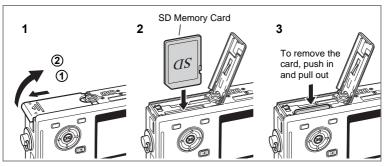
An SD Memory Card can be used with this camera. Captured images are recorded on the SD Memory Card if a card is inserted or in the built-in memory if no card is inserted.
