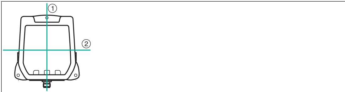
Figure 5.2 ① = vertikäl polarization plane ② = horizontal polarization plane
