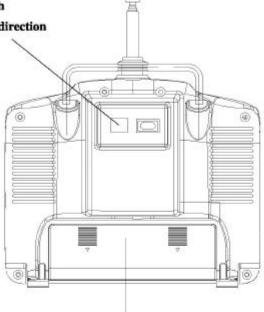
Battery Case's Cover Take out the battery case 's cover. Please use eight 1.5V dry battery or eight 1.2V NC battery. While setting battery, take care the polarity of the battery.
