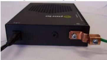
Attach the grounding lug to one end of an 18-12 AWG wire. 1.
