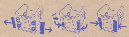
Insert 4 x C-size batteries using the + – symbols as shown.
