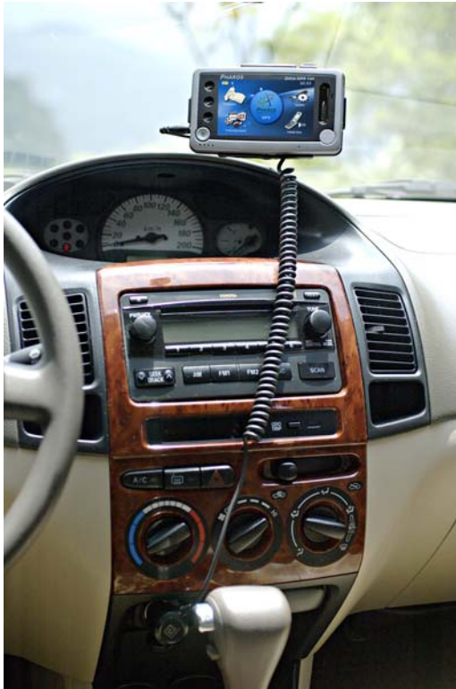
Figure 6: Power cord plugs into lighter
