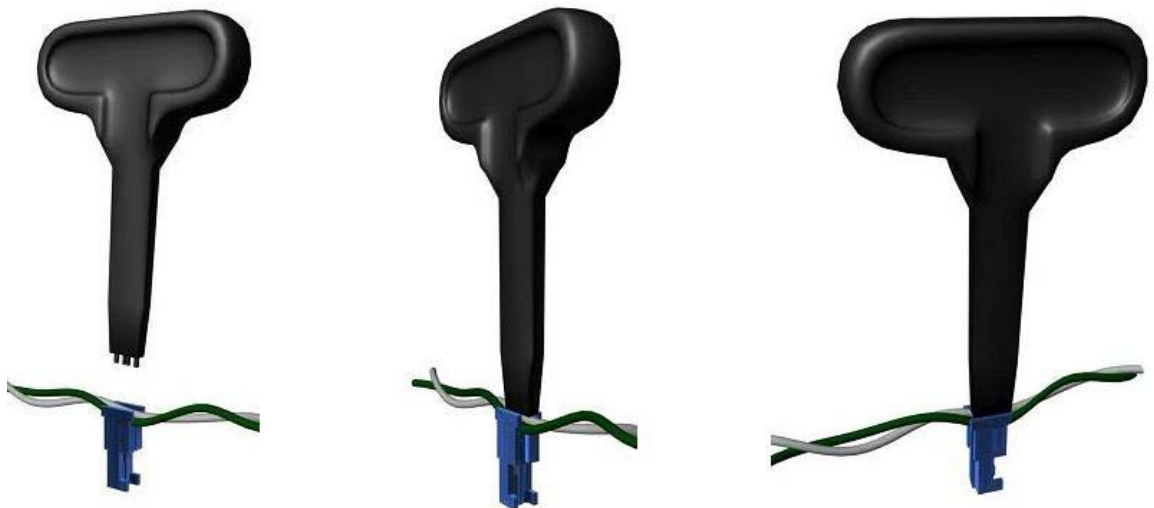
Figure 2.1.3: Attaching of connector to LED cable using crimp tool
