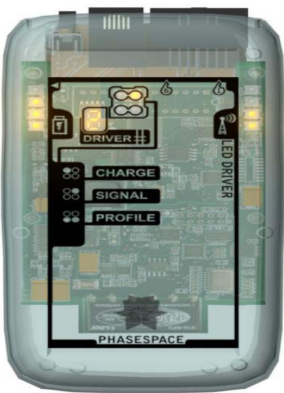
Figure 1.2.1: LED Driver Unit
