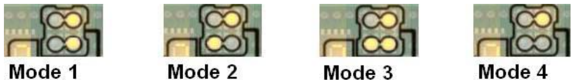
Figure 1.2.4: Mode indicator states
