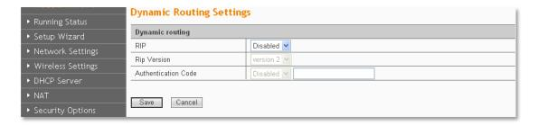
**RIP:** The Routing Information Protocol (RIP) is a dynamic routing protocol used in local and wide area networks. Choose **Enable** dynamic routing need to be activated.
