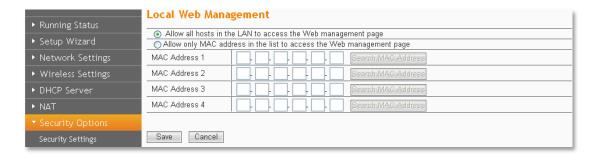
By default, the router allows all computers in the LAN to log in to the router for Web management. If you select **Allow only MAC addresses in the list to access the Web management page**, and add MAC addresses to the list, only MAC addresses in the list can access the web management page of the router, while other computers in the LAN are blocked from accessing the router.
