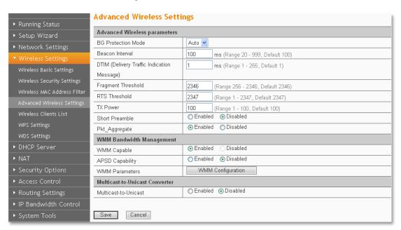
This section is to configure the advanced wireless setting of the Router, if you are not familiar with the setting items in this page, it's strongly recommended to keep the provided default values, otherwise it may result in lower wireless network performance.
