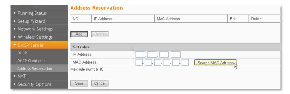
When you specify a reserved IP address for a PC in the LAN, that PC will always receive the same IP address each time when it accesses the DHCP server. Reserved IP addresses could be assigned to servers that require permanent IP settings.
