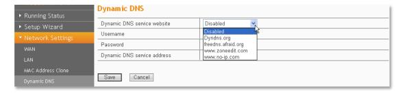
**Dynamic DNS** lets you assign a fixed host and domain name to a dynamic Internet IP address. If you want to use this feature, please register for this service with DDNS service providers such as www.no-ip.com first.
