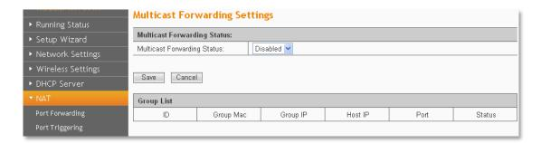
Multicast Forwarding enables the router to issue IGMP host message on behalf of hosts that the router discovered through standard IGMP interfaces.
