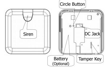
The multi sound siren PSE02 is a wireless siren, based on Z-Wave<sup>TM</sup> technology. Z-Wave<sup>TM</sup> is a wireless communication protocol designed for home automation, specifically to remotely control applications in residential and light commercial environments. The technology uses a low-power RF radio embedded or retrofitted into home electronics devices and systems, such as lighting, home access control, entertainment systems and household appliances.
