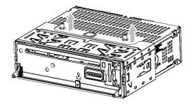
4 Remove the mounting sleeve with the removal keys.
