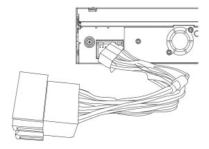
• If necessary, do the other connections. (See the last step in section **Connect** wires: ISO connector)
