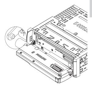
**3** Press the right side of the panel toward the left and point the hole to the pillar on the right.
