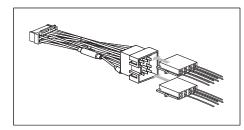
2 Connect the other end of the supplied standard connector to the unit.
