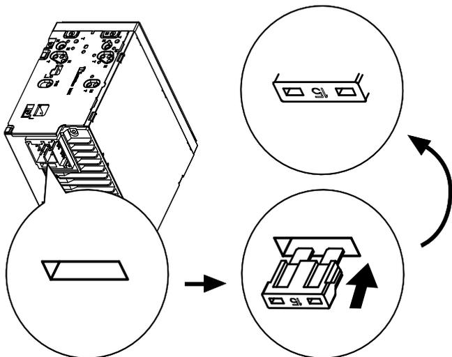
If the fuse gets damaged immediately after it has been replaced, there may be an internal malfunction. In such case, consult your Philips dealer.
