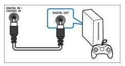
Using a coaxial cable, connect the COAXIAL connector on your SoundBar to the COAXIAL/DIGITAL OUT connector on the TV or other device.
