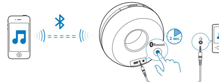
**EN** If SB3700 is connected through Bluetooth and an MP3 link cable at the same time, music should play through Bluetooth. To play through the MP3 link cable, switch off Bluetooth on SB3700 by pressing the Bluetooth button for more than two seconds. The Bluetooth indicator is off.
