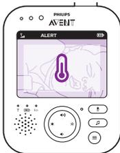
5 The parent unit shows this warning when chosen temperatures are measured.
