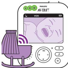
When your baby cries, the display and sound of the parent unit switch on immediately. The sounds are transmitted to the parent unit and the sound level lights turn green. As long as no sound is detected, the sound level lights are off
