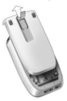
2 Place the batteries in the battery compartment.
