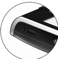
**Tip** Always switch off the Control Panel during transport to avoid activation of the touchscreen and the battery draining.
