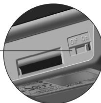
**Tip** Always switch off the Control Panel during transport to avoid the activation of the touchscreen and battery draining.
