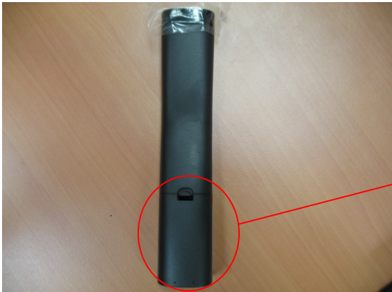
Picture 3: Remove the battery lid by pressed the hook down the battery lid and lift it up.
