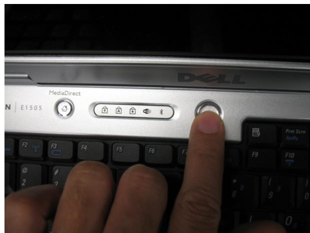
Picture 7: Press the switch to turn on the notebook.
