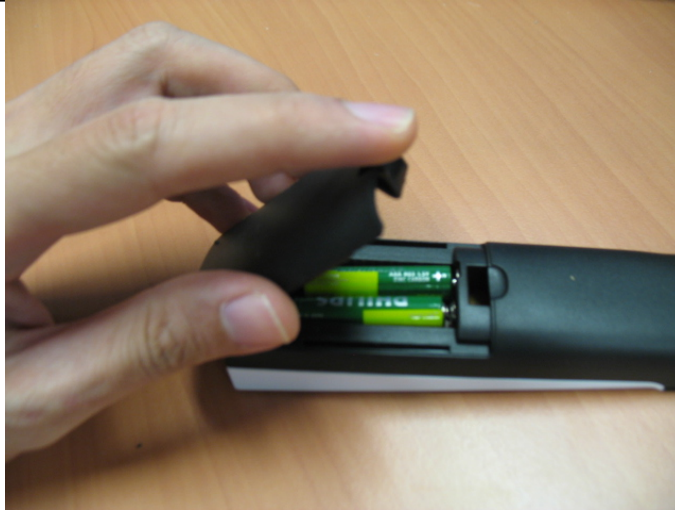
Picture 5: Closed up the battery compartment with battery lid.
