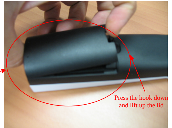
Picture 3: Remove the battery lid by pressed the hook down the battery lid and lift it up.
