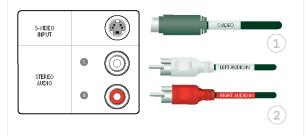
If your TV does not have a Component Video input, the S-Video connection will provide the best video connection for a standard- definition television.
