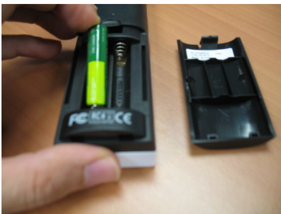
Picture 4: Insert the batteries (AAA type) with correct polarity.
