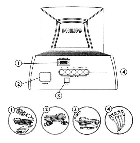
D-Sub Port - Attach the D-Sub connector that comes with your monitor here. Other end connects to your PC.
