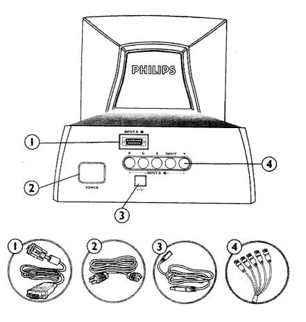
D-Sub Port - Attach the D-Sub connector that comes with your monitor here. Other end connects to your PC.
