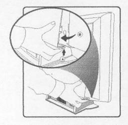
1) To remove the back cover, press up to disengage the clips on each side, then pull and lift.
