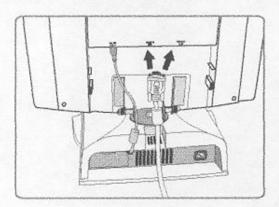
3) Plug in the video cable into VGA or DVI-D connector.
