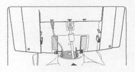
4) Cover the cables with the plastic ring and put the ring back on the hinge
