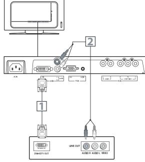
Digital Satellite Receiver with DVI connector
