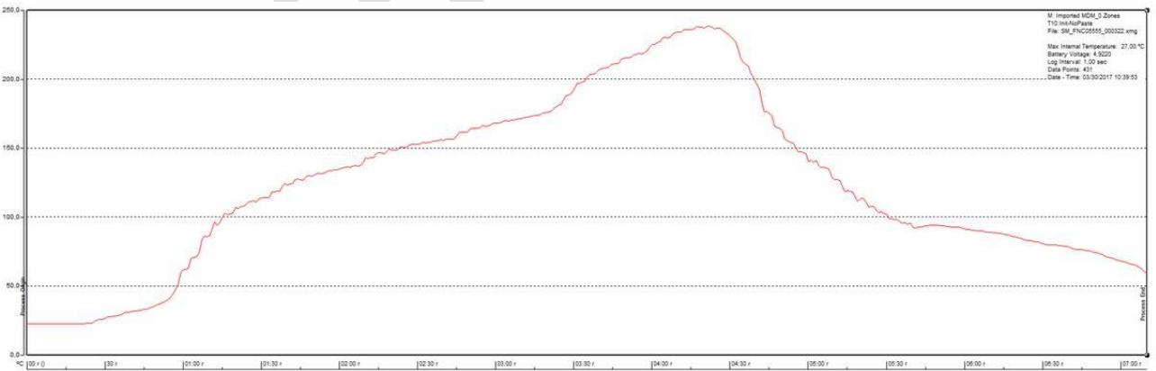
Figure 12: Reflow profile during test runs
