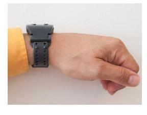
Recommended position of the wristband sensor skin conductance electrode for best results.
