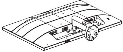
2. Hold the monitor base stand with both hands and firmly insert the base stand into the base column.
