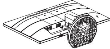
2. Press the locking clips to detach the base stand away from the base column.
