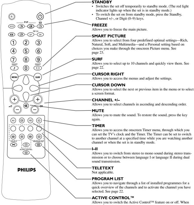
Allows you to switch the Active Control<sup>TM</sup> feature on or off. When Active Control<sup>TM</sup> is on, it measures and corrects all incoming signals to provide the best picture-quality settings, controlling Sharpness and Noise Reduction continuously and automatically. The onscreen Active Control<sup>TM</sup> display items cannot be selected. See page 21.
