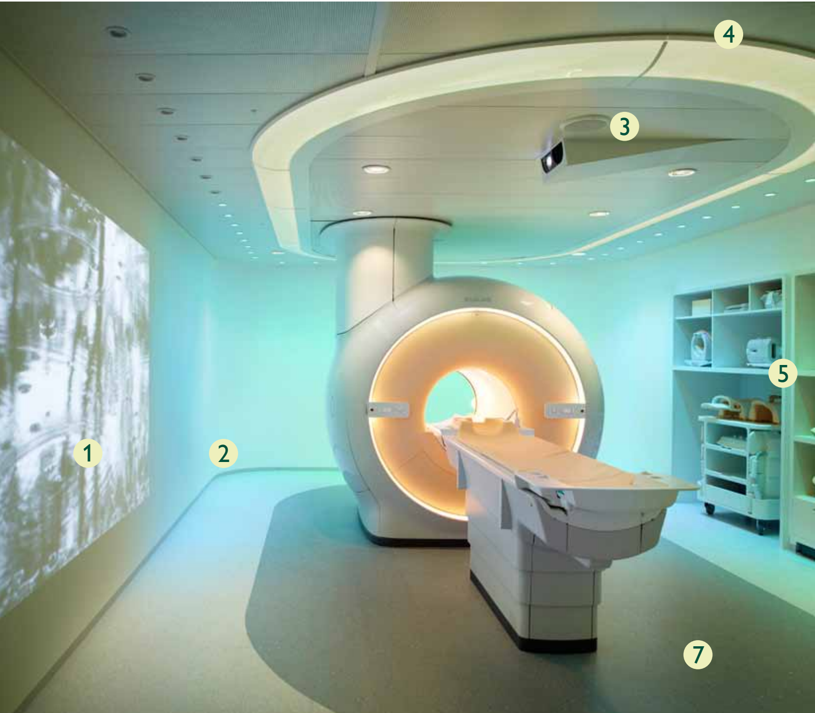
1 Side wall projection, 2 rounded corners, 3 audio system, 4 ceiling lighting element 'Halo', 5 integrated coil cabinets, 6 dynamic LED 'Ambient Lighting', 7 floor island
