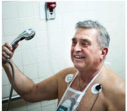
The IntelliVue MX40 withstands accidental drops from 1 meter (3.3'). It can also be temporarily immersed in water, including patient showering.
