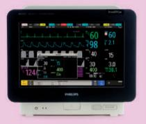
**IntelliVue MX500/MX450** includes an ambient light sensor, which automatically adjusts screen brightness to maintain readability in nearly any lighting – especially the low-light of the NICU.
