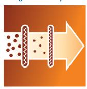
The two stage filtration system ensures that, once inside, the dirt cannot escape again. The first filter blocks most of the dirt, while the second filter traps the finer dust particles.
