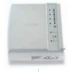
The IntelliBridge EC40 (4 data ports) or EC80 Hub (8 data ports) detects the device, and selects the right interface to capture its Medical Data Interface Language (MDIL) data. The hub then passes the data on to the IntelliBridge Device Interfacing Engine.
