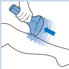
A Keep the flash button pressed. The appliance releases one flash after another as long as the safety ring is in full contact with the skin. Immediately after the appliance has flashed, slide the appliance to the next area. Make sure the safety ring is fully pressed onto the skin.
