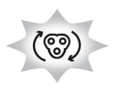
The latest Philips shavers have an inbuilt replacement reminder in the form of a shaving unit symbol. This symbol will light up and indicate you when to replace shaving heads.
