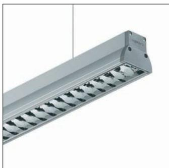
ThinMark TPS580 suspended luminaire with high-gloss optic with 3D micro-lamellae (C8) or very high-reflectance 3D micro-lamellae (C8-VH)
