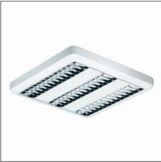
X-tendolight TCS398 surface-mounted basic luminaire with TL5 fluorescent lamp(s) and OLC high-gloss high-quality aluminum optic with 3D lamellae (C6)
