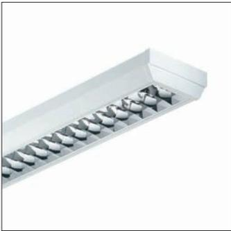
Finess TCSI98 surface-mounted luminaire with OLC high-gloss high-quality aluminum optics with 3D lamellae, limit 1000 cd (C6-1000 cd)
