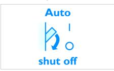
The electronic safety shut-off automatically switches the iron off when it is left unattended or tips over.
