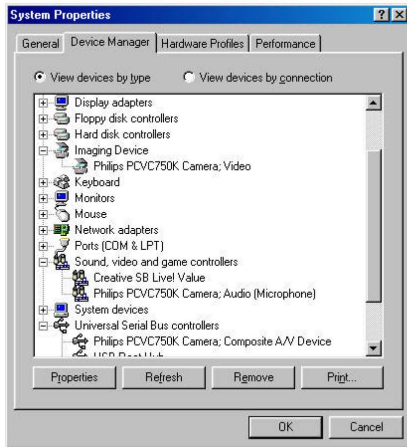
Let's look at USB for instance: an icon with the name 'Universal serial bus controller' should be visible. Click on this icon and Windows will tell you if this part of your computer system is operating correctly. Similarly, FireWire and other controllers can be checked.
