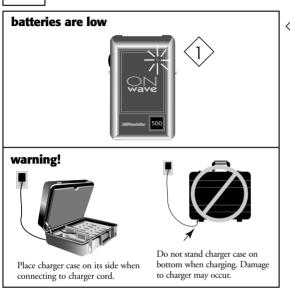
Light flashes when 2 hours of battery life remain (4 hours with alkaline battery)
