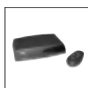
AT0801 aux-box (adds four additional audio inputs)
