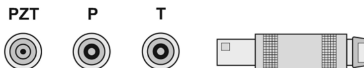
Figure 15: LEMO connectors: PZT, P and T
