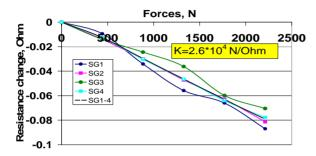
Figure 2: Calibration of bullet's SGs at T=290K.
