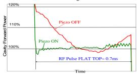
Figure 7: Forward RF power during CCII closed loop "flat top" at  $E_{Acc}$ =26MV/m. The red line shows forward power signal when Fast Tuner is OFF and the green line when Piezo is ON.
