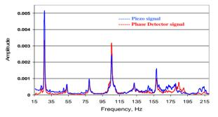
Figure 8: Frequency spectrum of cryo-flow induced vibrations in CCII.
