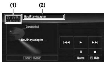
If you connect a Bluetooth adapter (e.g. CD-BTB200) to this unit, you can control a Bluetooth audio player via Bluetooth wireless technology. For details concerning operation, refer to the Bluetooth adapter’s operation manual. This section provides brief information on Bluetooth audio player operations with this unit that slightly differs or is cut short from the operations described in the Bluetooth adapter’s operation manual.
