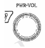
**POWER-VOL:** Push this knob to turn the audio system on and off. Turn this knob to adjust the volume. The system turns on in the last mode used.
