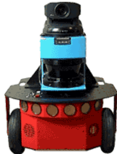
Figure 6. All ActiMedia robots may be configured with a variety of integrated accessories, including (DX shown here) a very high-performance laser range-finder and robotic pan-tilt-zoom color camera with onboard PC and framegrabber for color-tracking and surveillance.
