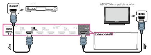
• Even if your set-top box is equipped with an HDMI output terminal, in some cases the sound is output from the digital audio output (optical or coaxial) and only the video is output from the HDMI output terminal. In this case, make the HDMI and digital audio connections as shown below.
