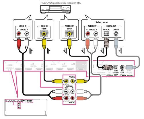
In order to record, you must connect the analog audio cables (the digital connection is for playback only) (page 67).
