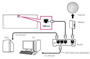
Connect the LAN terminal on this receiver to the LAN terminal on your router (with or without the built-in DHCP server function) with a straight LAN cable (CAT 5 or higher).
