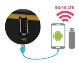
For increased WAN diversity, plug in a USB LTE modem as backup. Peplink routers are compatible with over 200 modem types. You can also tether to smartphones running Android 4.1.X and above. Compatible with: MAX 700, HD2 (all variants except IP67), HD4 (All variants)
