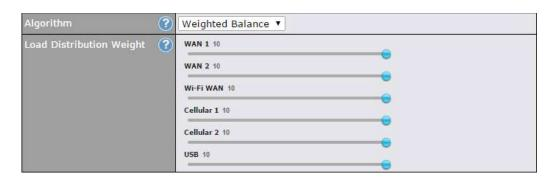
The amount of matching traffic that is distributed to a WAN connection is proportional to the weight of the WAN connection relative to the total weight. Use the sliders to change each WAN's weight.
