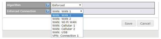
Matching traffic will be routed through the specified WAN connection, regardless of the health check status of the WAN connection. Starting from Firmware 5.2, outbound traffic can be enforced to go through a specified SpeedFusion<sup>TM</sup> connection.
